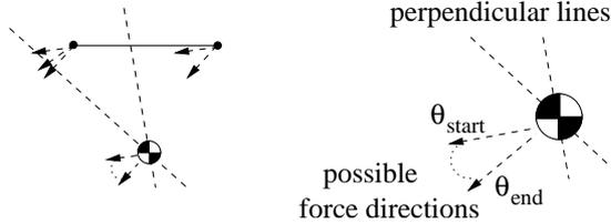
Fig. 4. A third value of  $\theta$  must be tested for the left endpoint because the extra  $\theta$  value is perpendicular to  $\phi$  and within  $[\theta_{start}, \theta_{end}]$ .
