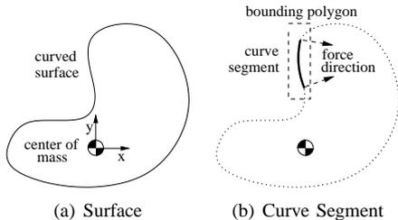
Fig. 1. The part is shown on the left. On the right a curve segment from the shape, the bounding polygon surrounding the segment, and the unit force vectors at the endpoints are shown.
