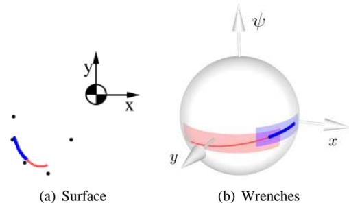
Fig. 7. Two curve segments along a surface are shown in the left figure. In the right figure the frictionless wrenches and bounds are mapped onto the unit sphere.
