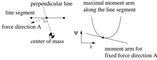
Fig. 3. The left shows a line segment with force direction A, the right shows a graph of moment for all maximal force directions and for the fixed force direction A
